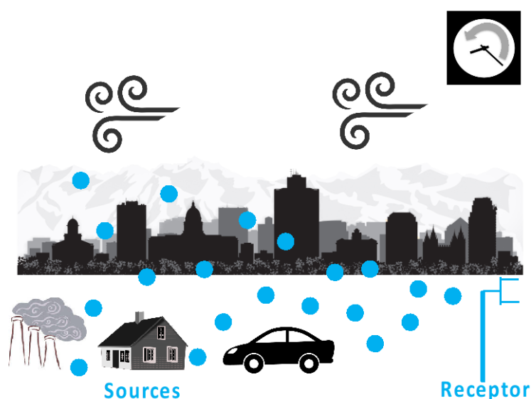
Figure 10: Application of Lagrangian particle dispersion model (LPDM) to link the receptor (where GHG measurements take place) to upwind sources by simulating the transport of an ensemble of air parcels backward in time. Turbulent dispersion is modelled through the stochastic motions of the parcels. The atmospheric “footprint”, or source-receptor relationship, is calculated by the amount of time the air parcels spend near the sources, typically at the ground surface.
