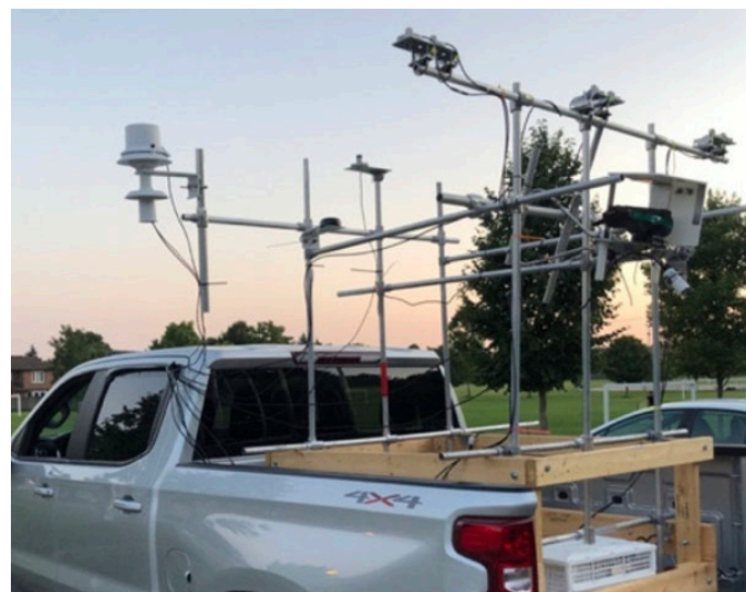
Figure 1. MTM set-up with instruments measuring air temperature, humidity, location, surface temperature, and incoming radiative fluxes.
