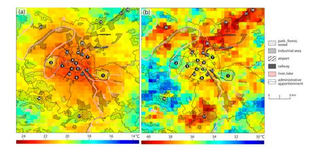
Figure 11. Satellite remote-sensing of land surface temperature. Land surface temperature composite images of the Paris region during the August 2003 heatwave (1 km resolution – National Oceanic and Atmospheric Administration Advanced Very High Resolution
