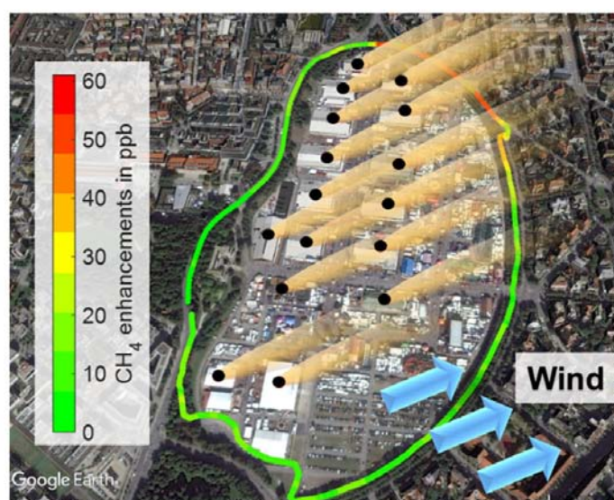
Figure 2: CH 4 enhancements around the Oktoberfest premises for two different wind directions (top: 20°, bottom: -110°). The highest enhancements can be observed downwind of the festival (Chen et al. 2020).
