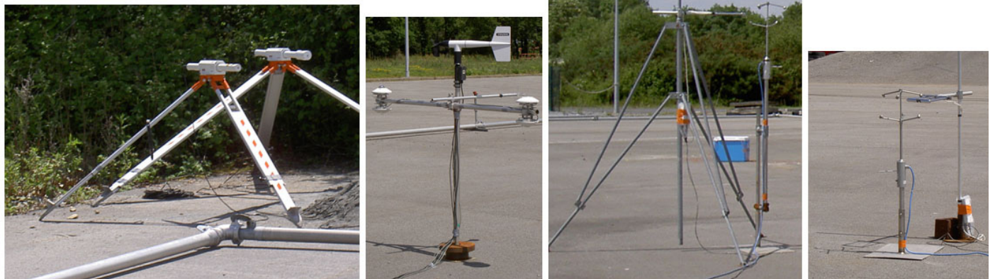
Figure 1. (a) View of the experimental site during a simulated rain event (the north is on the right); (b) zoom on some of the instruments. From left to right: small aperture scintillometers, radiation and wind sensors, 3D sonic anemometers and Krypton hygrometers at 2 m and 1 m.
