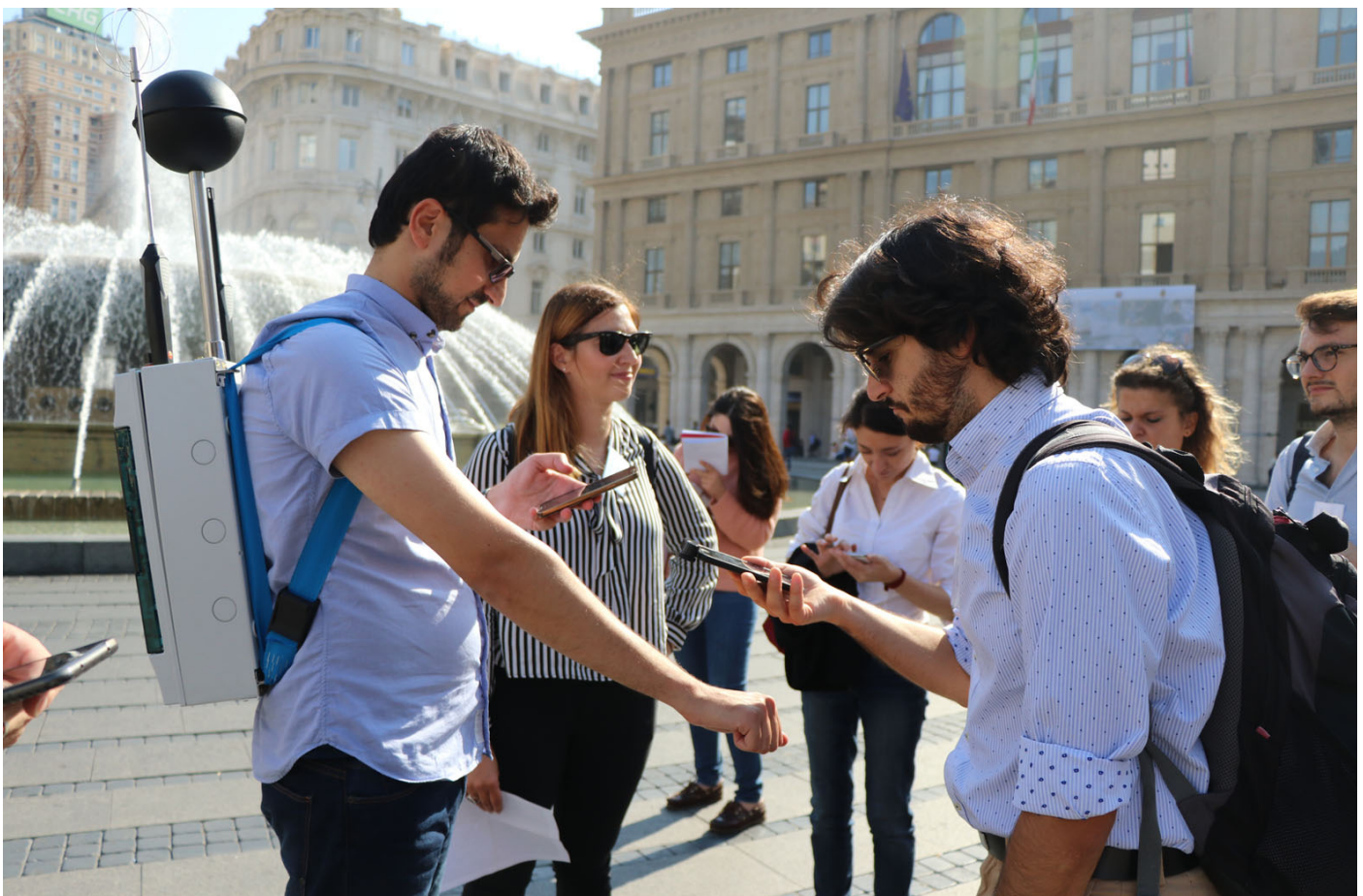
Figure 4. Measurements by portable weather station with globe thermometer, and infrared thermocamera.
