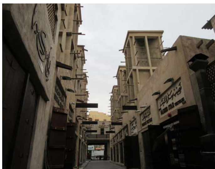
Down an alleyway in one of Dubai’s many souks (a street market formed by a narrow maze of alleys lined with open-air storefronts). Buildings in older parts of town often have rooftop windtowers (called “Al Barajeel”, pictured) to aid ventilation. Photo by James Voogt.
