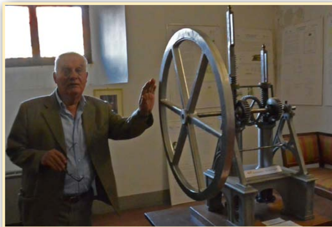
One of the rare artifacts housed in the observatory is a model of the world's first internal combustion engine , invented in the mid-19th century by Barsanti & Matteucci and reproduced some 150 years later by Renzo Macii (left).
