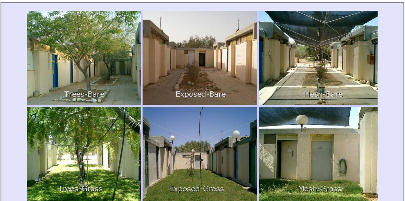
Figure 3. Courtyard setup with various combinations of overhead shading and ground cover.
