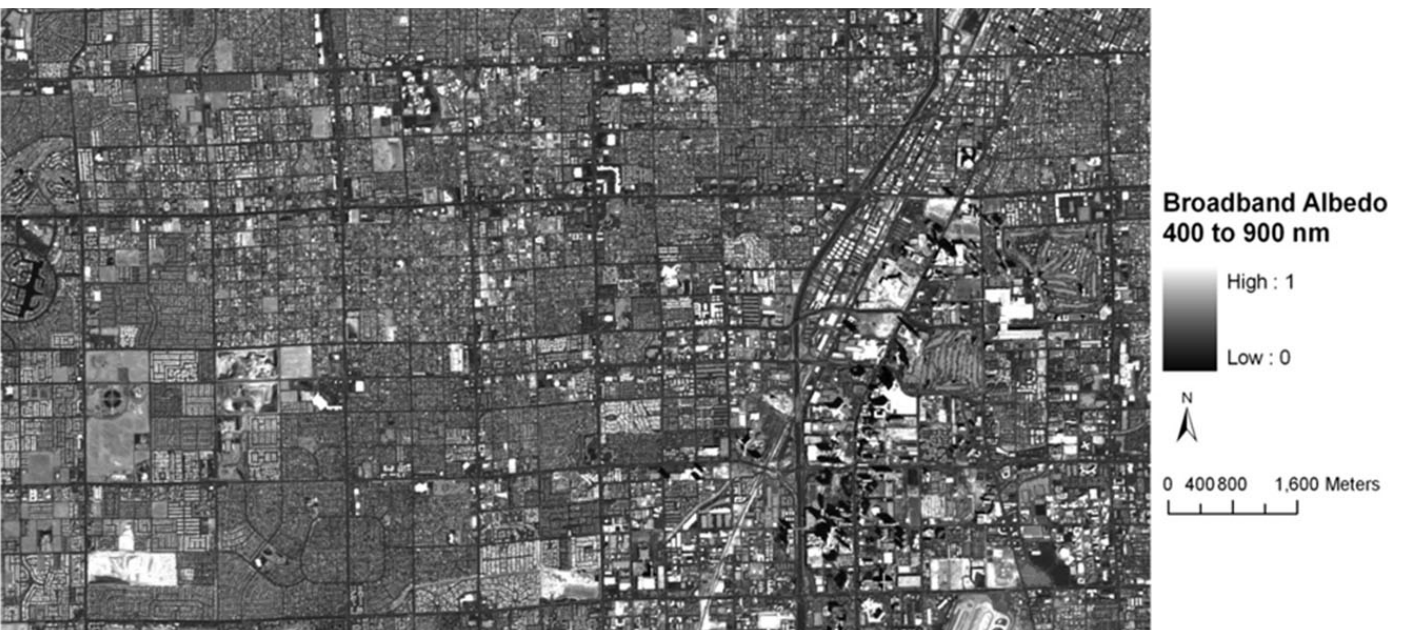
Figure 5. Broadband albedo map of the Las Vegas study area, using the VNIR/Surf model.
