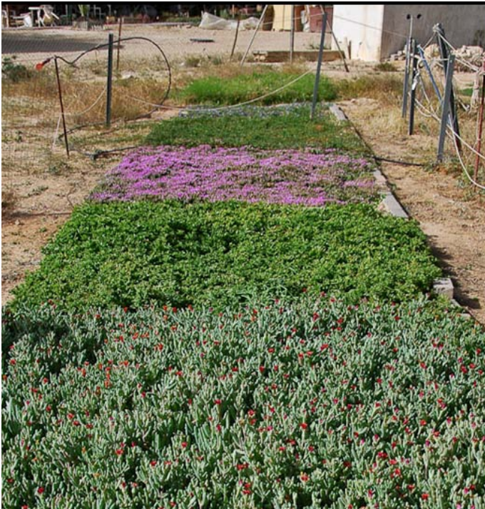
Figure 7. Planted experimental plots for measurement of surface albedo and radiative surface temperature.
