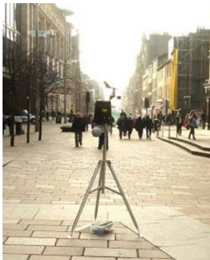
Figure 3. 'Mobile' weather station (Davis Vantage Pro2) with gray globe thermometer.
