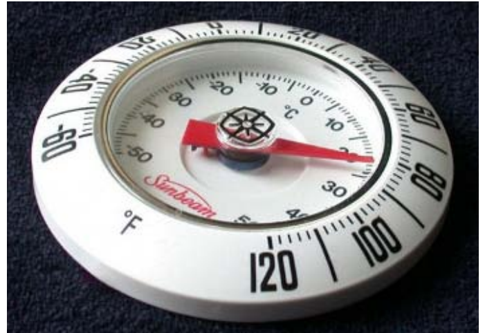
Bimetallic coil thermometer. Source: Inside Science
