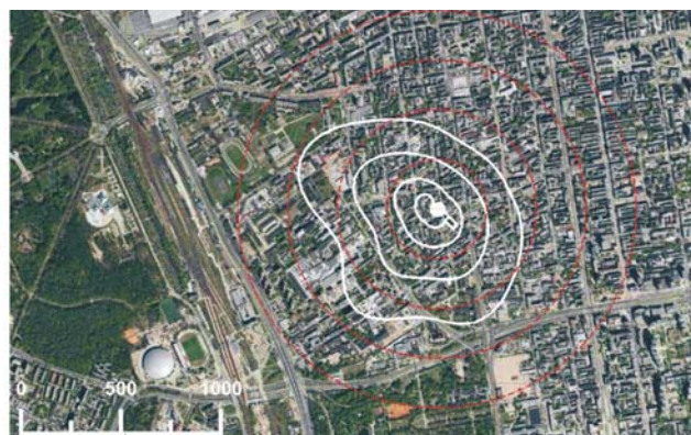
Figure 1. Locations of CO 2 flux measurement in Łódź (left: L - Lipowa Street, R - residential area, I - post-industrial area, A - airport, suburban area) and the surroundings of the Lipowa measurement point (right). Solid white lines indicate source areas at P = 50%, 75% and 90% calculated for unstable stratification (all available data in the period July 2006-April 2011). Map and aerial photo source: Municipal Center of Geodesics and Cartographic Documentation of Łódź.
