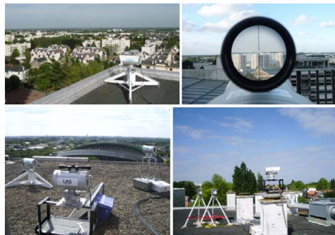
Figure 5. Setup of scintillometers on high building roofs.
