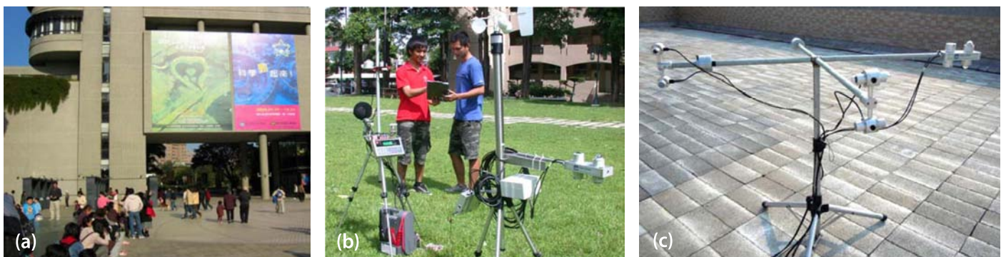
Figure 1. Photos of locations of field experiment in Taichung (a) and Yunlin (b). The T_{mrt} is evaluated both by the globe thermometer and the six-direction short- and long-wave radiation measurement station (c).
