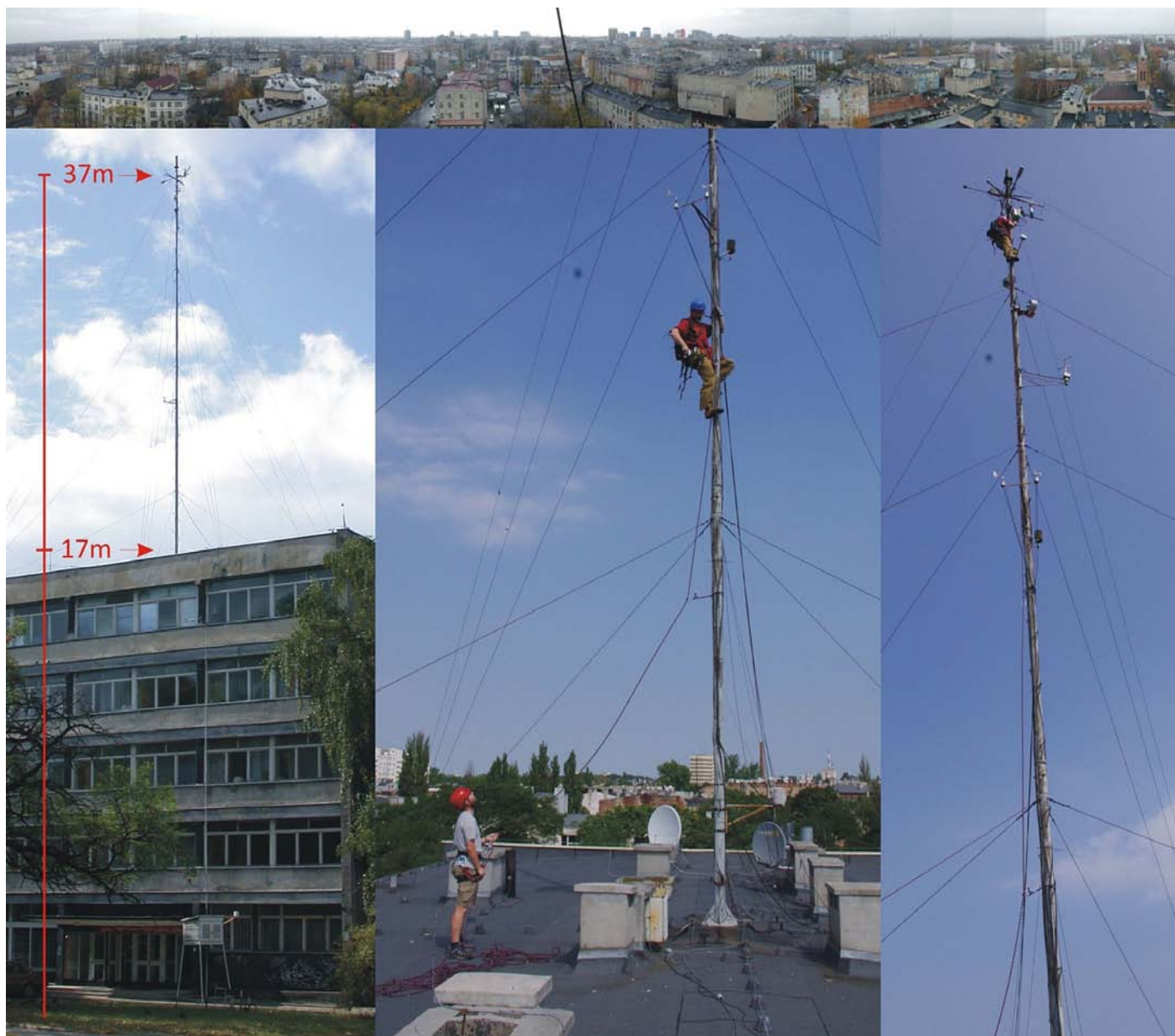
Figure 2. Urban canopy around the Lipowa measurement site (top), and measurement tower at Lipowa Street (bottom, with sensor maintenance shown at middle and right). Photo: K. Fortuniak.
