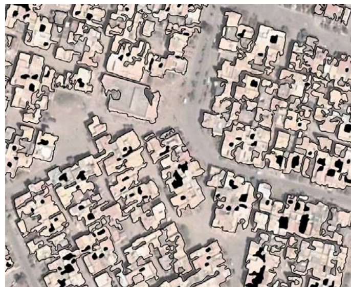
Figure 6. Recognized buildings and courtyards overlaid on original image - output of GIS classification process
