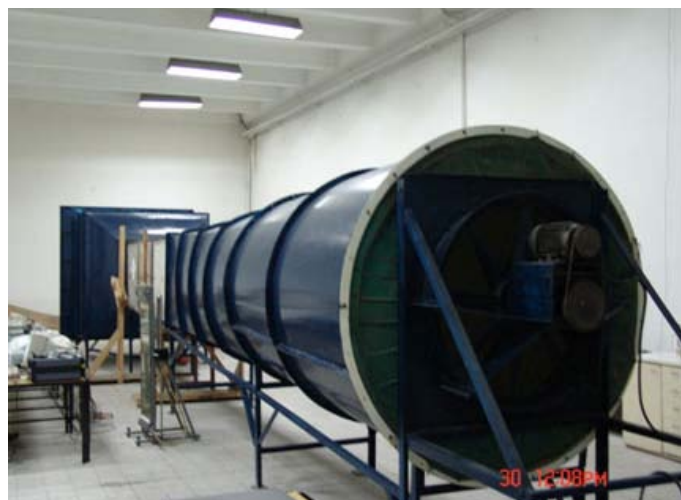
Figure 1. Wind tunnel of Physical Environment Control Laboratory of Faculty of Architecture. Air entry to the tunnel is provided by a bell-mouth of 250x250x0.30 m. Two flow-shaping modules are of 2.00x2.00x0.92 m in section. Square-section observation module of 1.05x1.05 m connects flow shaping module with an adaptor of 1.30 m in length. An axial type fan has been mounted to the other side of the tunnel. The engine has a power of 1.5 kW and has a period of 1450 pulse/sec.
