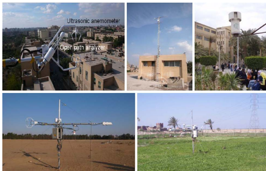
Figure 1. Upper left and middle: The eddy covariance tower at Cairo University. Upper right: Sigma-2 Sampler at Cairo University. Down left: 10th Ramadan station. Down right: Bahteem station.
