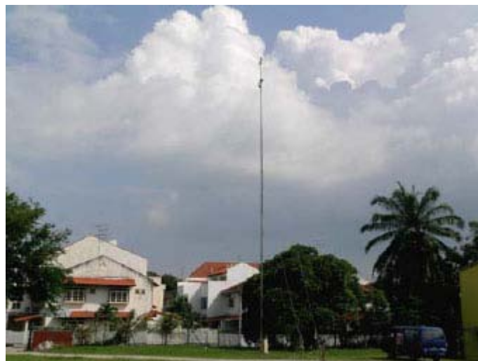
Figure 3. Pneumatic micrometeorological tower with eddy covariance sensors installed at 20.7 m above ground.
