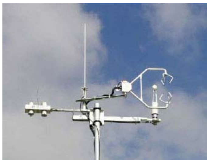
Figure 4. Close-up of eddy covariance sensors installed at top of mast. CSAT3 and Li7500 are visible on r.h.s. and CNR1 on l.h.s. Thin vertical extension in center is lightning rod.
