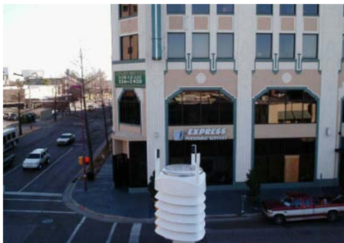
Figure 3. View of the WXT510 sensor associated with the traffic light station installed at the intersection of Main St. and Walker Ave. in Oklahoma City (looking south at the elevation of the sensor; sensor height is approximately 10 meters).
