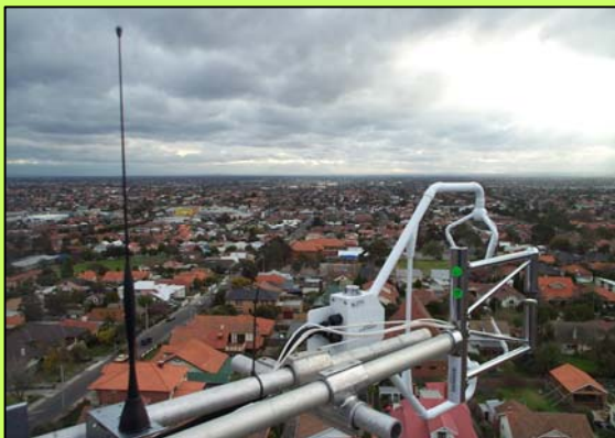
Figure 2. Eddy covariance system at the Preston site established August 2003. CO 2 fluxes were also conducted at this site in February 2004.
