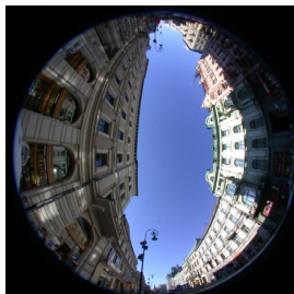
Fig. 4 Total (left) and UV (center) radiation measured on the roof level (with an unobstructed sky view) and in the urban canyon with a sky view factor of 0.424 and H/W ratio of 1.1 in Łódź. On the left is an upward bird eye picture from the canyon measurement point (Podstawczyńska, Pawlak, 2003).
