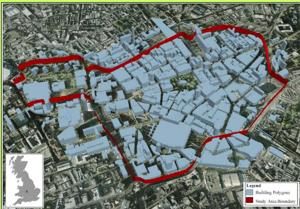
Figure 2 3D scene of Birmingham CBD showing extruded polygons from which \psi_s can be calculated (adapted from Studden, 2007)
