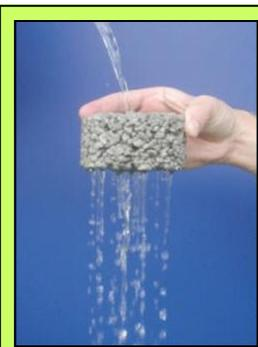
An example of pervious concrete. Source: [www.concreteparking.org/images/](http://www.concreteparking.org/images/)
