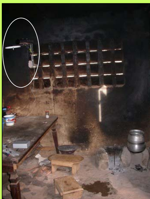
Figure 4. Instruments (encircled) mounted in a wood fuelled kitchen. The simple stove on the floor to the right in the picture, Apart from the entrance doorway, the only ventilation is via the holes in the wall seen in the picture.
