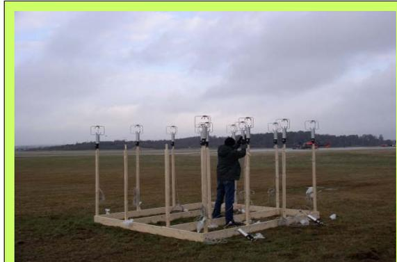
Figure 2a. Performing an inter-comparison of the sonic anemometers prior to field observations.
