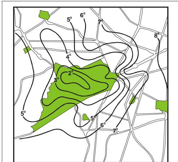
Figure 3: Isotherms in Chapultepec Park on December 3, 1970 (5:28 to 6:48), with clear sky and calm air. Redrawn from [5].
