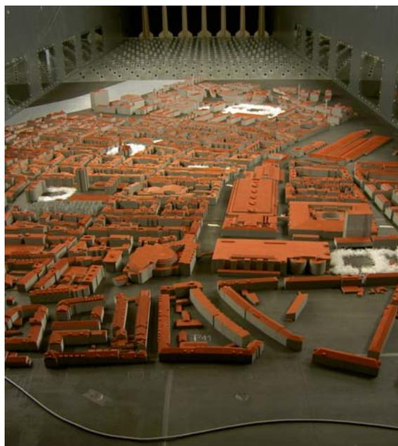
Fig. 2: Physical model in the wind tunnel of the University of Hamburg (scale 1:300) of that region in the City of Basel, where intensive observations had been performed in the field (white background in Fig. 1).
